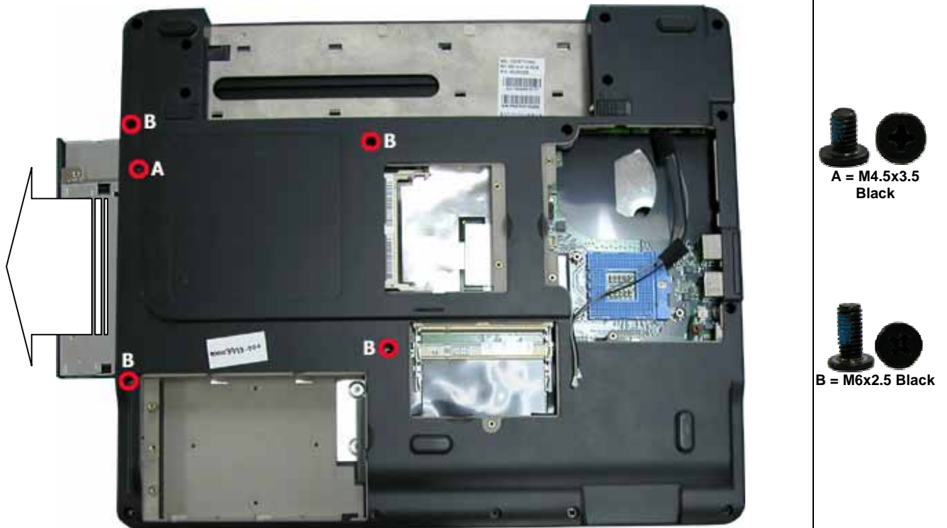
Fig. 13 Releasing the optical drive
